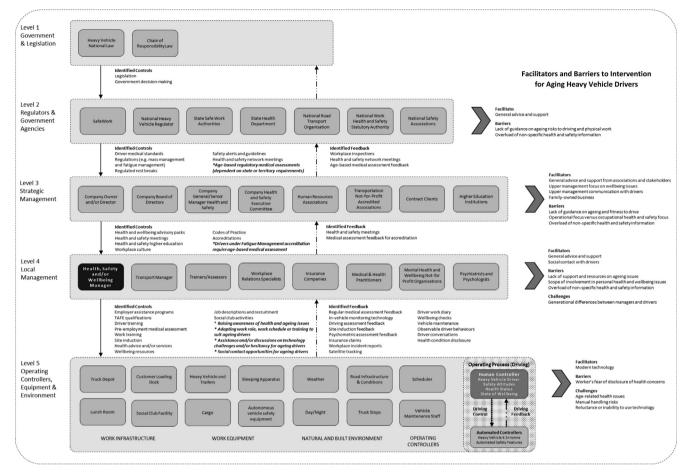
Fig. 1. STAMP Control Structure of Health, Safety, and Well-being Interventions for all Heavy Vehicle Drivers as Identified by Organizational Managers (\* Age-specific interventions as identified by managers are presented in **bold italics**).
