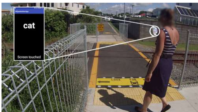
Fig. 3. Illuminated in-ground LEDs; participant equipped with eye-tracking glasses and performing the visual distractor task.
