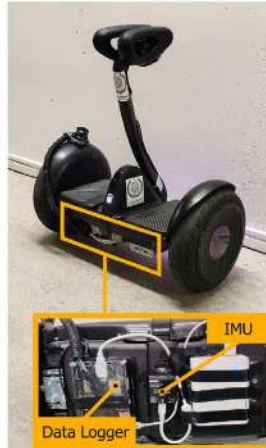
Fig. 1. Instrumented vehicles with data loggers and inertial measurement units (IMUs).
