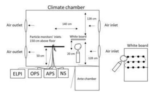
Fig. 1. Climate chamber and spray scenario setup. ELPI = Electrical Low-pressure Impactor, OPS = Optical Particle Sizer, APS = Aerodynamic Particle Sizer, NS = NanoScan (Scanning Mobility Particle Sizer).
