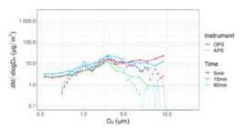
**Fig. 4.** Particle size distribution over time of the mass concentration of Product#5. The particle size distribution at 5 min, 15 min, and 60 min is plotted for both OPS and APS.
