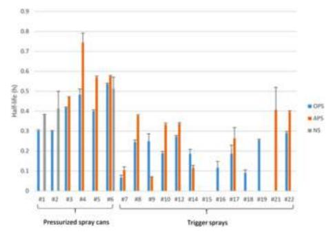
**Fig. 3.** *Half-life times* of the decay of the total particle *mass* concentrations released by 19 spray cleaning products, six pressurized spray cans (Product#1–6), and 13 trigger sprays (Product#7–22). Product# is shown on the x-axis. Error bars are the standard error of mean (SEM) of the *half-life times*.
