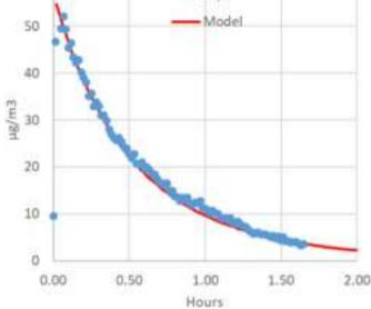
Fig. 7. Comparison of experimental OPS data for total particle mass concentrations with ConsExpo predicted decay. The data is from the pre-test of Product#3.
