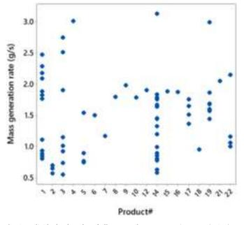
Fig. 2. Individual value plot of all measured mass generation rates (MGRs) at low doses of 19 spray cleaning and disinfection products.
