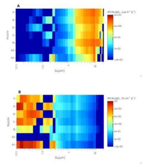
Fig. 5. Heatmap of 10-min average of NS, OPS, and APS normalized *mass* (A) and *number* (B) concentration particle size distributions of the 6 different nozzles sprayed with the same product (Product#14). The two entries for the original nozzle are for two different bottles (showing differences in particle distributions for the same product and nozzle).
