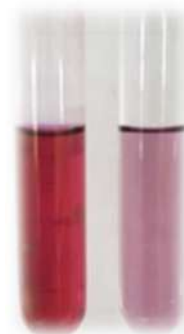
Fig 8. The color change from wine red (AuNPs-AHMT) to purple (AuNPs-AHMT-Cortisol)
