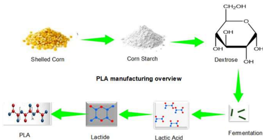
Fig 1. Overview of the production of PLA
