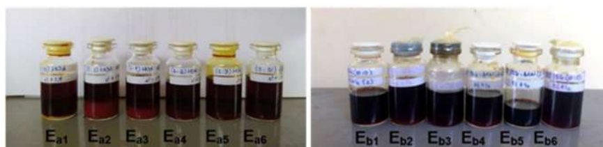
Fig 4. KI/I 2 electrolyte with acetonitrile:DES a3 (left) and acetonitrile:DES b4 (right) as solvent
