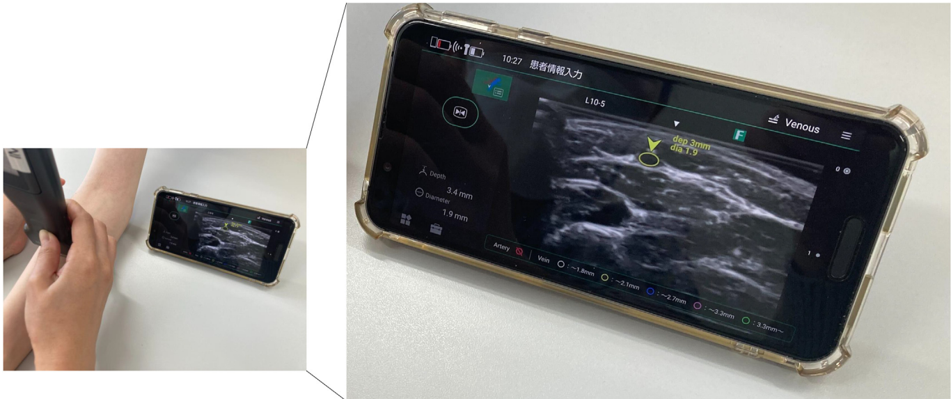
Figure 2. An Ultrasound System with An Automated Vessel Detection System Using Artificial Intelligence. The system detects areas that have characteristics of a vessel (circular or ellipsoidal anechoic area) and displays the vein size and depth in real time.
