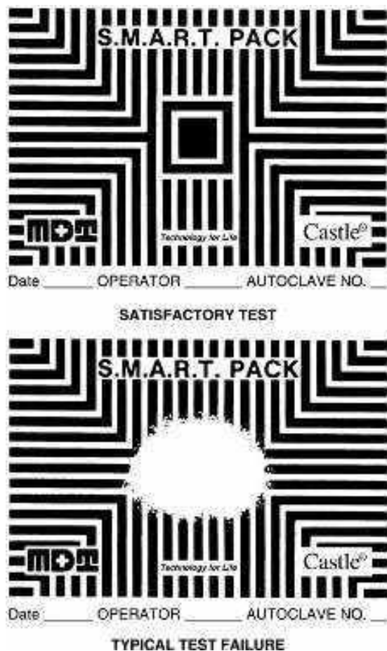
Figure 3-19 Air removal test. Courtesy of MDT Biologic Company, Rochester, NY.
