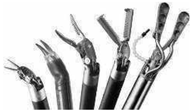
Figure 8-22 DaVinci robotic instruments. © 2015 Intuitive Surgical, Inc. Used with permission.
