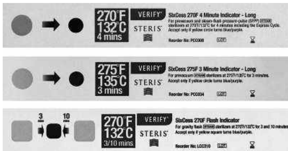
Figure 3-11 Class Six emulating indicators are designed for specific steam sterilization cycles: (A) 270°F/132°C 4 minute cycle (B) 275°F/135°C 3 minute cycle (C) IUSS 3 and 10 minute cycles. Courtesy of Steris Corporation, Mentor, OH.
