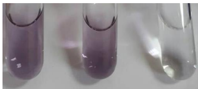
Figure 1. Qualitative Cyanide Test ( \text{CN}^- )
