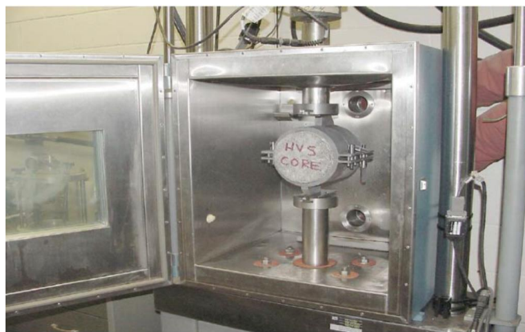
Figure 5. FDOT bond strength device (Sholar et al., 2004)
