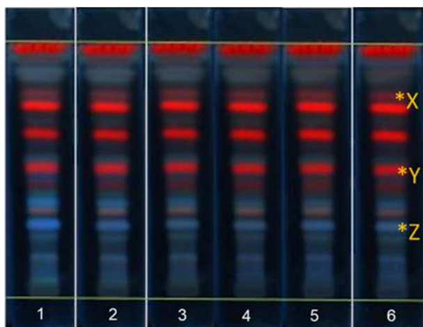
Fig 5. The TLC chromatogram of S. rhombifolia leaves extract after (1) 2 nd , (2) 5 th , (3) 10 th , (4) 20 th , (5) 30 th , (6) 60 th min using UV light 366 nm with the sulfuric acid derivatization reagent
