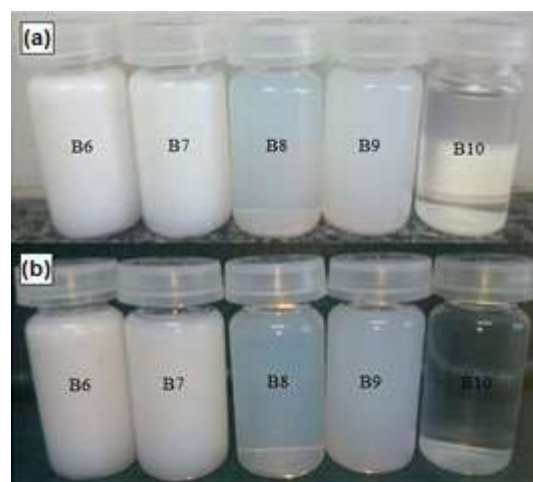
Fig 3. Nanoemulsions based on orange essential oil sample: (a) on first day, (b) after 20 days synthesis
