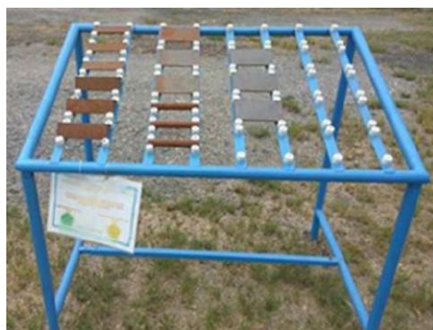
Fig 2. Test specimens on a test rack with samples exposure
