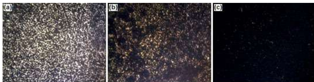
Fig 3. Light microscope images of ACC surfaces prepared with several carbon particle sizes using 80 wt.% adhesive: (a) 60, (b) 80, and (c) 100 mesh
