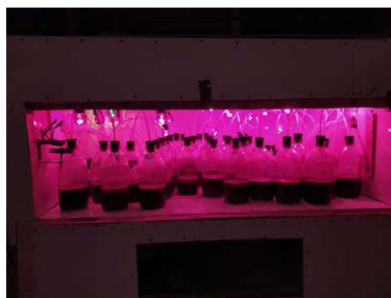
Fig 3. Biogas production under 55 °C
