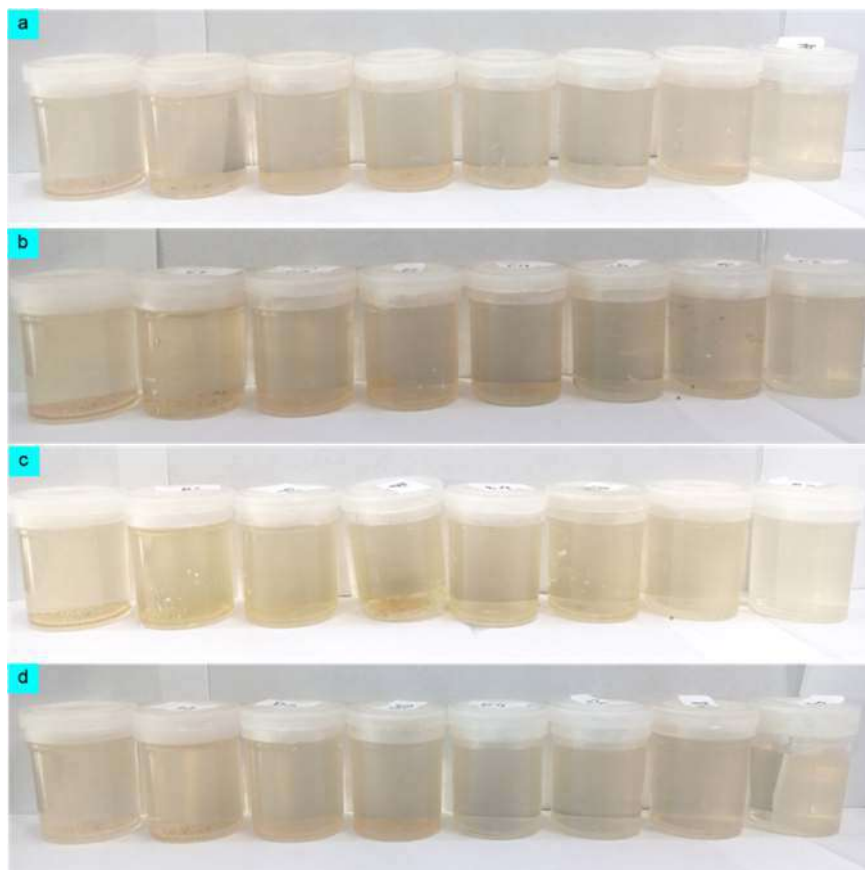
Fig 6. Images of Silau River water treated using (a) PVA/40TiO 2 /60SiO 2 , (b) PVA/60TiO 2 /40SiO 2 , (c) PVA/80TiO 2 /20SiO 2 , and (d) PVA/100TiO 2 /0SiO 2 for 1–8 h (from left to right)
